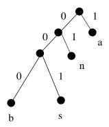
**Encoding:** For each character locate corresponding leaf and follow the path, adding 0s when going left and 1s when going right. bananas 0001011011001 (13 bits - wow!)
